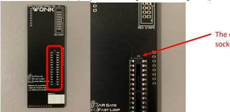
The dimple on the silkscreen and socket should be aligned
